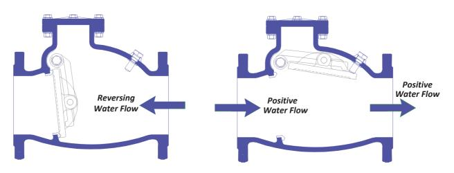
Swing Check Valve in closed position
